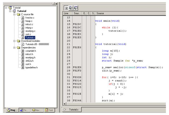
Figure 3.3 Editor window (displaying the source program)
